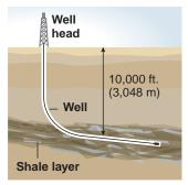
1. A well is bored using directional drilling, a method that allows drilling in vertical and horizontal directions to depths of over 10,000 feet (3,048 meters)
