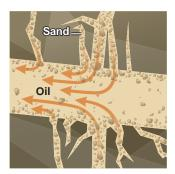
3. Sand flows into the fissures, keeping them open so that the oil from the shale can flow up and out of the well
